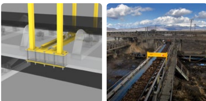
Installation on belt conveyor frame using clamps and bolts
